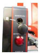
The range of the photocell is adjusted by a screwdriver (B).
