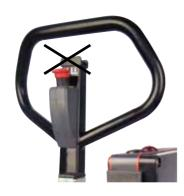
**NOTE!** Manual operating of the handle is not possible when the level control is active.
