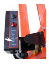
Upwards or downwards positioning can be chosen on the arrows (up/down).
