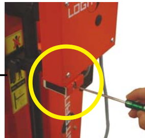
Adjustment of the detection range (of the photocell)
