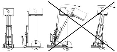
The Logiflex is designed for use on even and level floor. During transport the forks shall be raised as little as possible. Transport with raised forks should be made over the shortest possible distances and at low speed.
