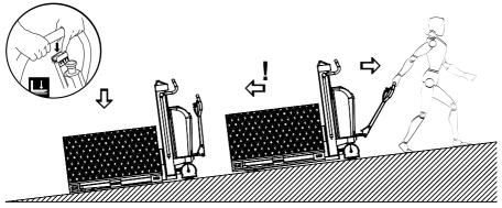
If it becomes necessary to use the load as a brake to prevent the Logiflex from running away, activate the DOWN button quickly, until the load reaches the ground.
