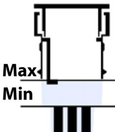
**Note!** Do not fill in distilled water to maximum level, until the battery is fully charged. The liquid level increases considerably during charging.
