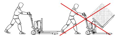
The Logitilt is designed for use on even and level floor. During transport the forks shall be raised as little as possible. Transport with raised forks should be made over the shortest possible distances and at low speed.
