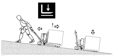
If it becomes necessary to use the load as a brake to prevent the Logitilt running loose, activate the DOWN button quickly until the load reaches the ground.
