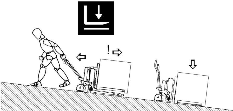
If it becomes necessary to use the load as a brake to prevent the Logitilt running loose, activate the DOWN button quickly until the load reaches the ground.
