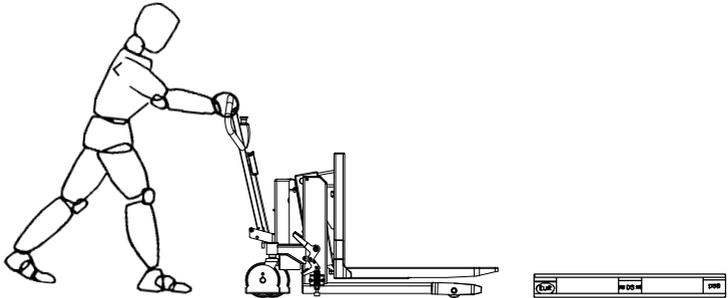
The Logitilt has assisted steering on one wheel to make manoeuvring easy.
