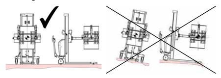
The load centre is never allowed to exceed the centre line of the wheels. During transport with load, the carriage shall be raised as little as possible. Transport should be made over the shortes possible distances at low speed.
