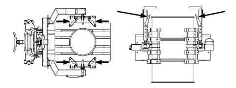
Clamp slightly around the drum, and lower the gripping arms (E), until the locking plate (C) locks at the edge of the drum.
