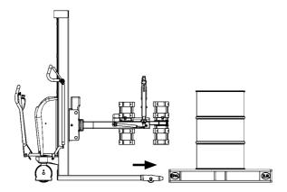
The height is adjusted, so that the clamps (A) are placed approx. 5cm above the middle of the drum, and the top lock (D) is moved to upper position.
